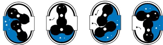
As shown in the picture, two contra-rotating impellers of two-lobe or "figure 8" design are encased within a rigid measuring chamber, with the inlet and outlet connections on opposite sides. Precision machined timing gears keep the impellers in correct relative position. Optimal operating clearances between the impellers, cylinder and headplates provide a continuous, non-contacting seal.
