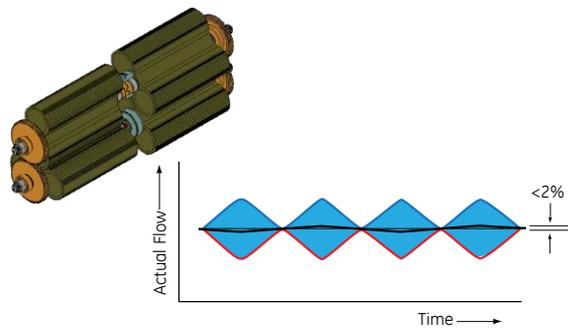
Fiorentini Twin rotary meters provide significantly improved accuracy over conventional rangeability make them ideal choices for reference or master meter applications. Reduced pulsations also significantly reduce ambient noise, making Twin rotary meters ideal for sound sensitive applications.
